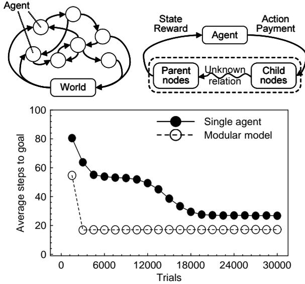
Fig 2: (Top) Schematic diagram of networked RL. (Bottom) Averaged learning curves for the task in Singh (1992).
