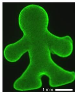
▲ Process living cells into micro beads, accumulate the beads to fabricate millimeter scale 3D tissues.
