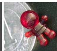
micro humanoid fabricated by micro stereolithography
