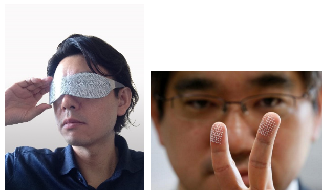
PrivacyVisor® protecting against facial detection and BiometricJammer preventing fingerprint capture
